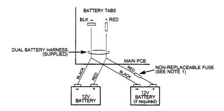
**Note 1:** This fuse is intended to prevent the risk of battery harness flame-out when two batteries are used and one battery is connected with proper polarity and the other is connected with reversed polarity. This fuse will not open circuit under any other condition. Observe proper polarity when making connections.
